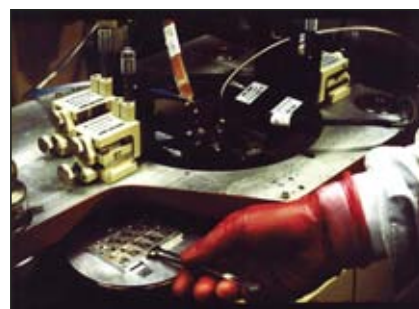
▲ Fig. 5 Fixtured MMICs being fed into an on-wafer test stand.
