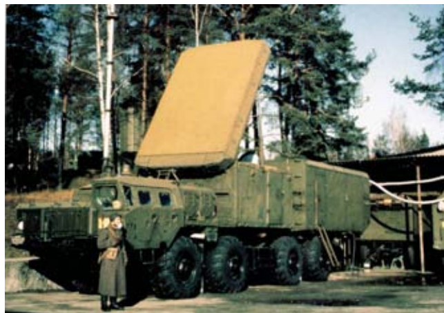
▲ Fig. 5 A 30N6-1 (NATO: Flap Lid) fire-control radar for the S-300 system. (Rosoboron export photo)
