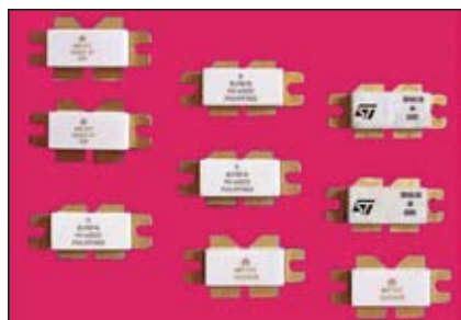
▲ Fig. 5 Some LDMOS transistors for applications up to 1 GHz.
