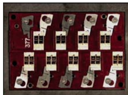
▲ Fig. 4 COBRA HPAs on carriers fixtured for RF test using on-wafer pulsed RF test equipment.
