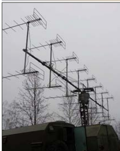
▲ Fig. 2 Yagi antennas of the P-18 Spoon Rest.
