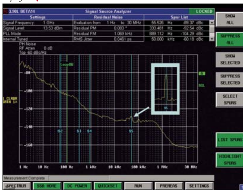
Fig. 1 A typical phase noise measurement using the phase detector method, with the signal frequency, level and residual noise displayed. ▼
